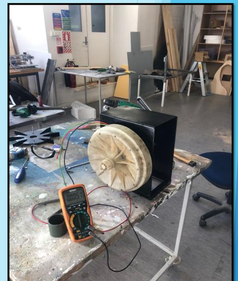
The testing the generator output
